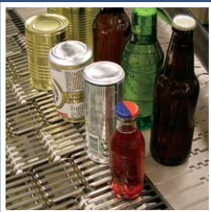
Rexnord® DTS®-C self-clearing DynamicTransfer System™ at infeed and discharge provides smooth product transfers.
